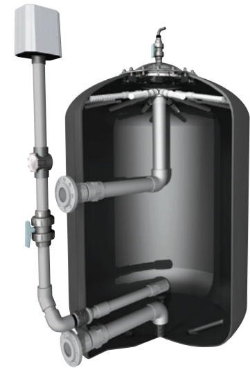
Inside View - XFM Fines Filter 1200
